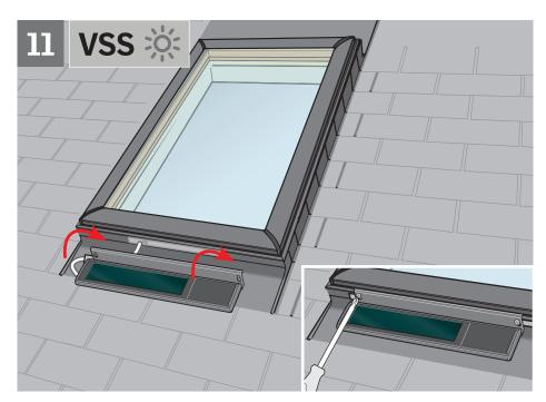
**ENGLISH:** After installing bottom and side flashing parts, install solar panel as shown and secure with screws.
