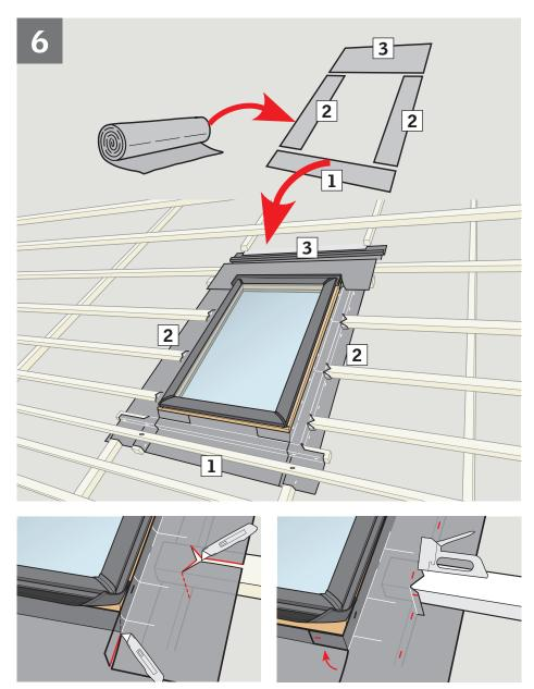
**ENGLISH:** If roofing underlayment is used: Dress roofing underlayment up around all four sides of the frame. Roof with counter battens shown for illustration purpose.
