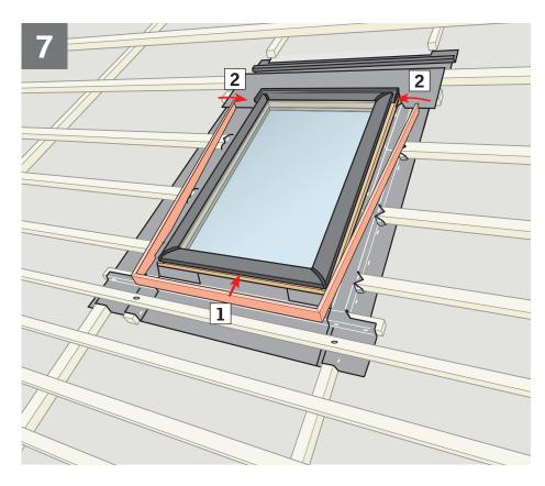
**ENGLISH:** If flashing is not to be installed immediately, replace the cladding parts starting at the bottom. Interlock side frame claddings with bottom frame cladding as shown. Secure the claddings with the original screws.
