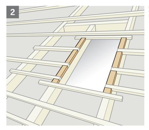
**ENGLISH:** Consider infill battens along the sides to reduce heat loss/improve thermal performance.
