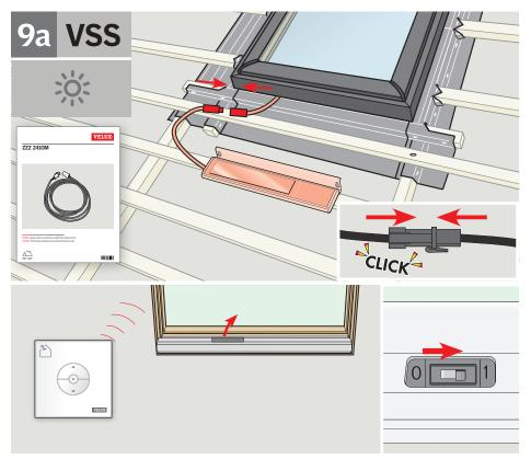
**ENGLISH:** Connect wire as shown and do not install the solar panel until the bottom flashing has been installed.
