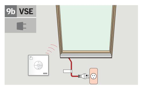
**ENGLISH:** Connect plug on power supply cable to approved electrical power outlet. The junction or outlet in/to which the skylight power supply cable is connected must be accessible for inspection when installation is complete.
